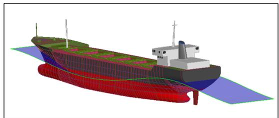
The buoyancy has been calculated from the Common Structural Rules as hydrostatic pressure:
