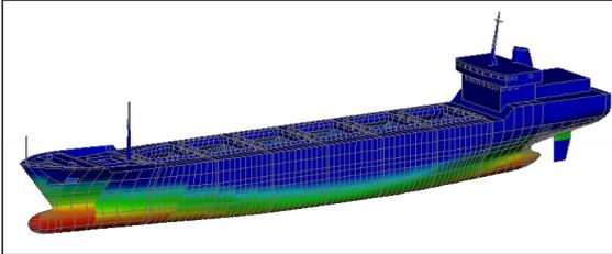
Despite the fact that a good balance was achieved, the resultant force and moment are not precisely zero. So in order not to have an unrestrained model that can cause problems with Nastran the Inertia Relief technique was used. In this way the resultant forces and moments are balanced by inertial forces induced by an acceleration field.
