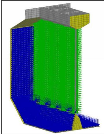
The self weight, meaning the weight of the element net, is 5487 tons. The mass of auxiliary structures that doesn't contribute to ships strength is assumed to be 4000 tons. This results to a tonnage of approximate 29800 tons. The corresponding waterline is calculated using this total weight, at a level of 11.3 meters above ships bottom, using the Tank Tool of ANSA.
