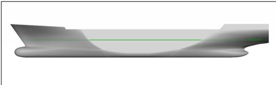
The center of buoyancy is calculated and used for the proper non structural mass distribution.
