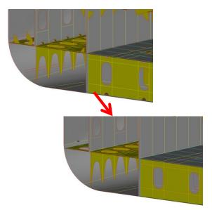
The model is almost 100% symmetrical with differences only in some openings in various plates, but since they do not play an important role in the current analysis, they can be neglected. Thus, half of the model can be deleted. This greatly reduces the pre-processing time since all the tasks are applied to half model. When the model is ready the other half is created with linked (children) symmetric entities.
