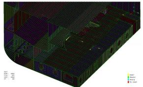
The profile parts can be exported by FORAN as beams or surfaces. In this case,
