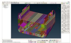
The profile parts are also translated as ANSA parts. In this approach, the additional information of the profile parts (scantling, section area, etc.) is attached to the ANSA parts as comments. Both the plate and profile parts carry the information of the block and ship that they belong to, as part attributes
