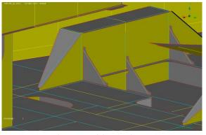
Among the additional numerous capabilities in handling geometrical features, holes and welding cuts can be automatically filled and cracks can be closed.
