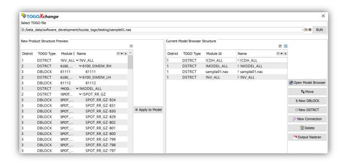
The tool reads .nas file with TOGO comments which describes the tree-structure and converts it to ANSA's Part/Group structure. It also lets the user to manage the tree-structure, create new TOGO entities with specific naming convention. The tool allows you to output the model with TOGO comments back into a NASTRAN file.
