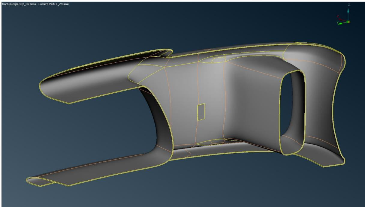
**Figure 2: Bumper CAD model (rear view) with patch antenna placed behind it**
