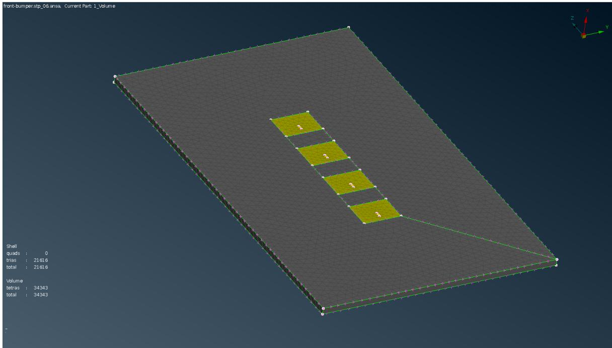
**Figure 1: Meshed CAD model of the patch array**
