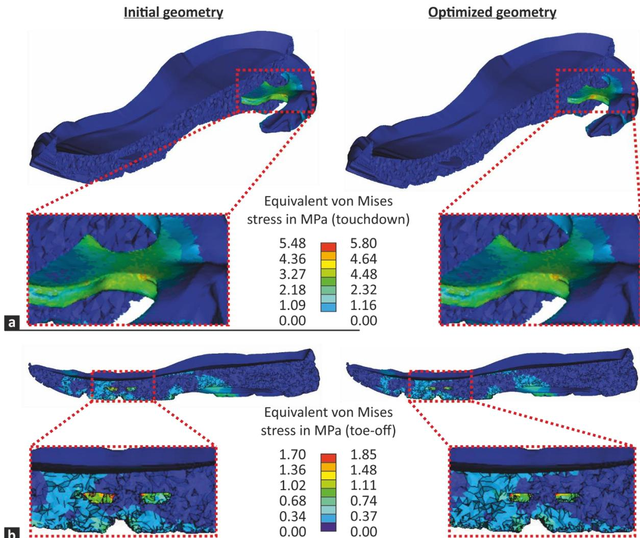
Figure 1 – Varying stress distributions in the initial vs. optimized gel-pad configuration, during: a) touchdown and b) toe-off.
