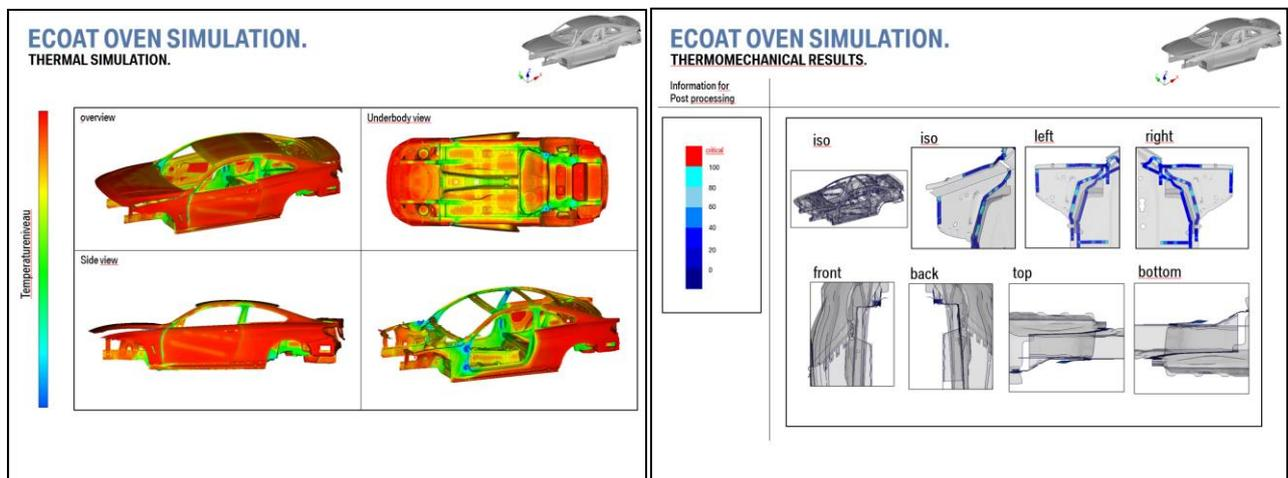
Figure 2 – Exemplary presentation of thermal and thermomechanical simulation results.
