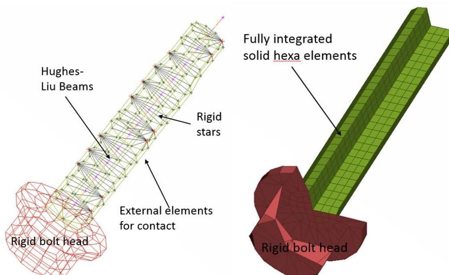
Figure 2 – Simple way of modelling bolts with beams and null solids for contact (Left). Corresponding new detailed solid hexahedron model (Right).
