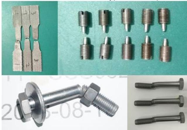
Figure 1 – Pictures of samples from quasi-static and high speed tension testing (upper), as well as bending and shear validation testing (lower).
