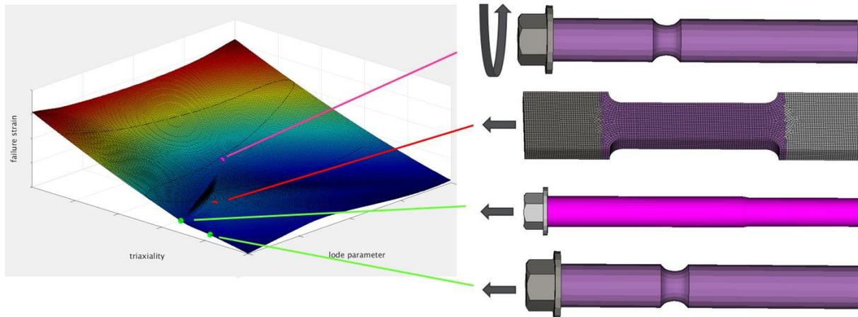
Figure 3 – A selection of the test setups that builds up the failure strain surface as function of stress state.
