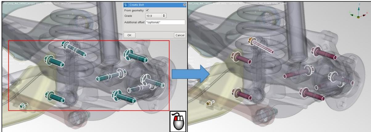
Figure 6 –Converting multiple CAD generated bolts in a rear suspension into detailed solid meshed counterparts, with a few clicks via the automatic bolt script toolbar. Correct attributes, material and pre-tension is also set by the script.
