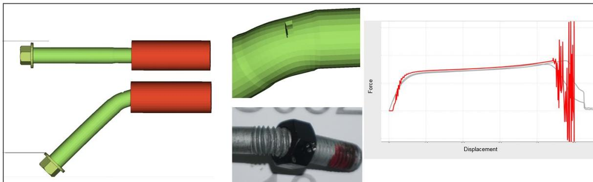
Figure 4 – Example of bending correlation testing (grey curves) vs replication in simulation (red curve).
