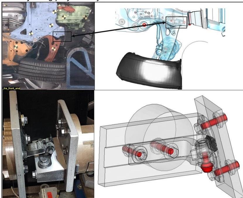
Figure 7 – Correlation of bolt model in small overlap (upper) and door hinges (lower).
