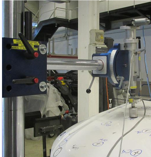
Figure 1- Ateca Bonnet in an experimental analysis.
