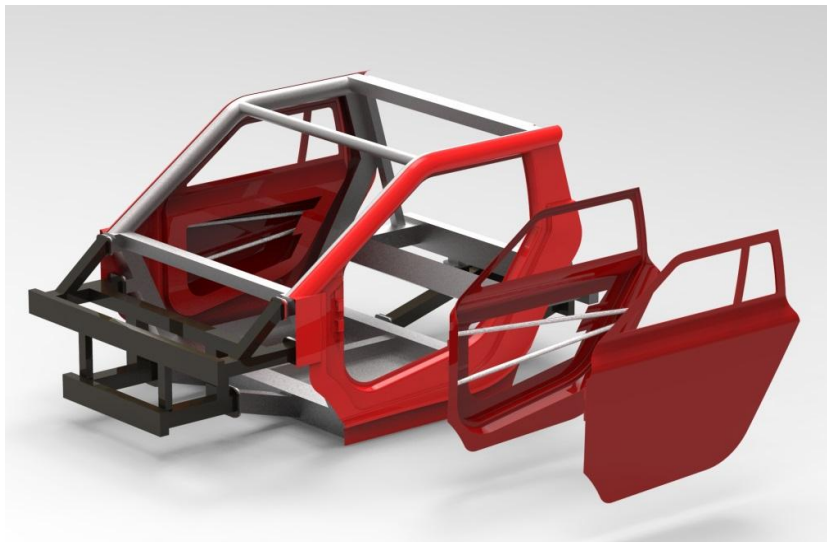
Figure 1 - Door components exploded view, as attached to vehicle chassis.
