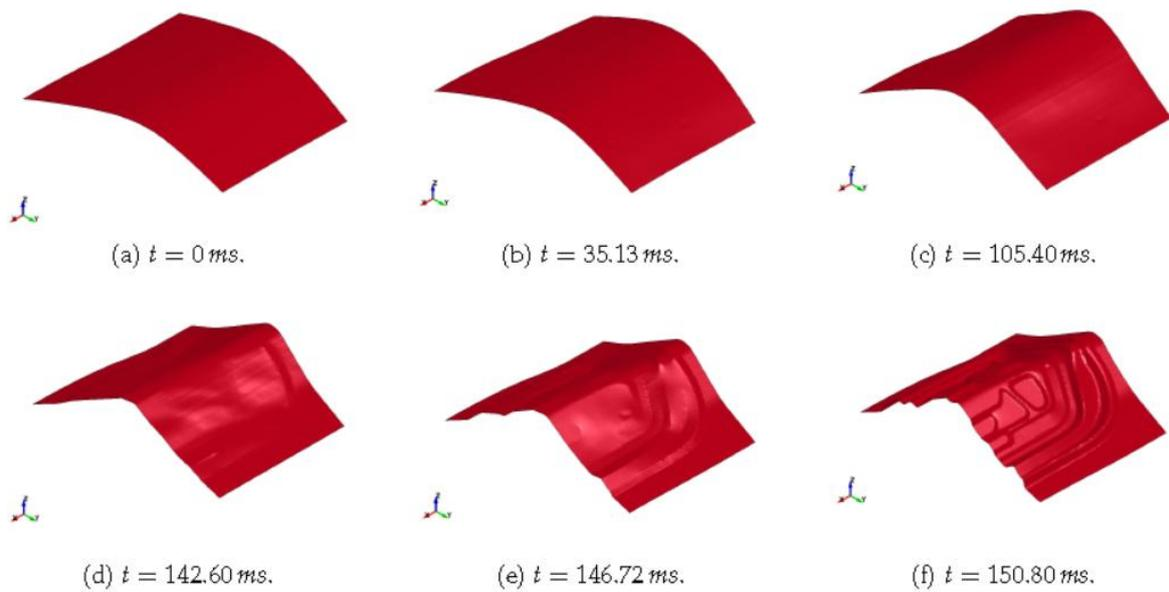
Fig. 9. Progressive decklid panel deep drawing
