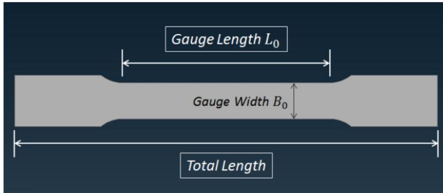
Fig. 1. Specimen dimensions
