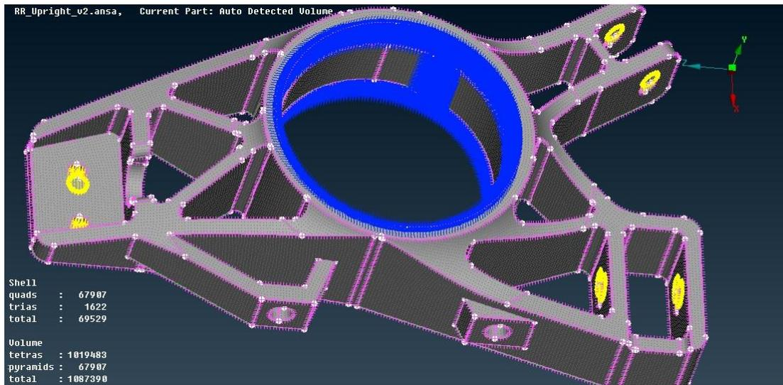
Figure 2 - Forces (yellow) applied on the surface of the holes – constraints applied on the bearings surface (blue)
