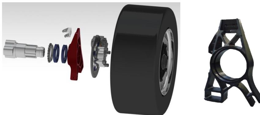
Figure 1 - Upright (red colour) position in the wheel (left), Rear Upright design (right)
