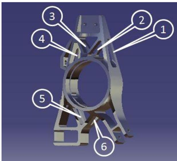
Figure 4 – Redesigned upright based on the topology optimization
