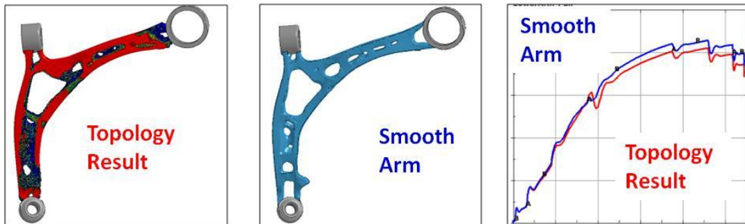
Fig.6: The topology results compared to the smooth arm structure as a result of manual post processing. The comparison of the force strokes curves is shown to the right.
