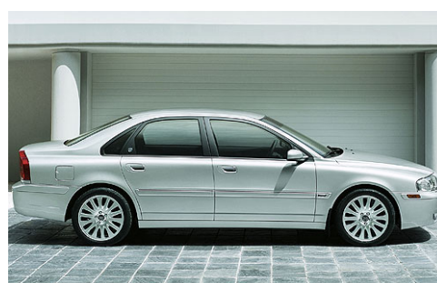
Photo courtesy of Volvo cars North America Coefficient of drag, Cd – 0.28 Gas mileage (combined) – 23 mpg†
