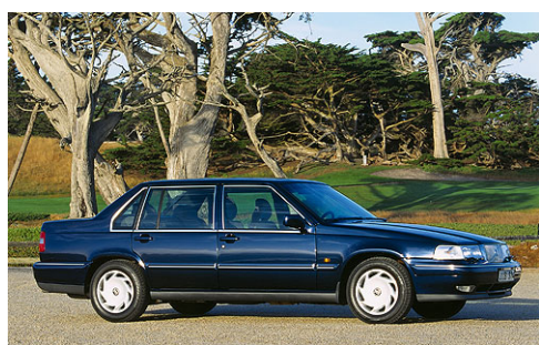
Photo courtesy of Volvo cars North America Coefficient of drag, Cd – 0.36 Gas mileage (combined) – 18 mpg†
