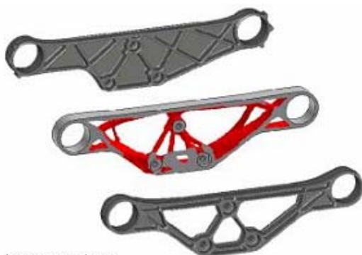
Fig. 2: Topology optimization example
