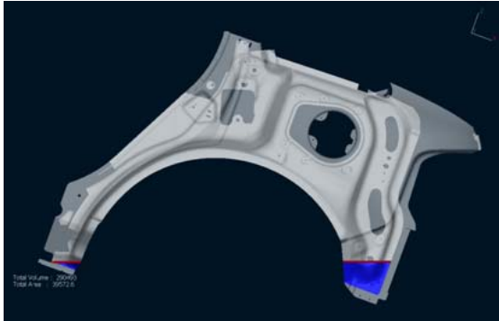
Figure 12: E-coat accumulation was identified by V.TRAPS.
